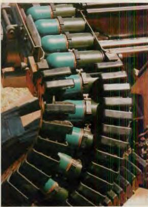
(top) When employed in the ground role, the Striker will usually be mounted on the M3 .50-caliber Browning machine gun tripod. Note the test-bed cradle interfacing the AGL with an M3 tripod. (above) The Striker's direction of feed can be varied from the left or right in the field by simply replacing the feed assembly. (left) When required, the Striker can operate reliably from a vertical position. The last-round hold pawl was designed for this purpose.
